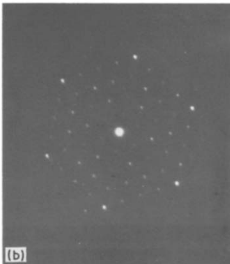
Figure 3 Yttrium oxide precipitate in the as-cast Ti-1.84% Y alloy electrodes: (a) dark-field image; (b) selected-area diffraction pattern of [111] pole; (c) schematic diagram of diffraction. (○) intense reflections, (●) weak reflections, (x) forbidden or very weak reflections.
